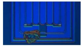
Wafer with debris: reflected light, C-DIC, EC Epiplan-APOCHROMAT 50x/0.95
