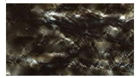
Silicon thin-film solar cell: surface of a thin-film solar cell; reflected light, polarized light; EC Epiplan-APOCHROMAT 50x/0.95
