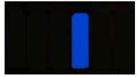
Hot stuck pixel: bright spot on black background caused by blue subpixel stuck in the "ON" state.
