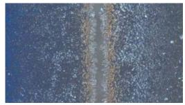
Laser edge isolation scribe: laser-textured edge isolation scribe on monocrystalline silicon solar cell; EC Epiplan-APOCHROMAT 20x/0.60
